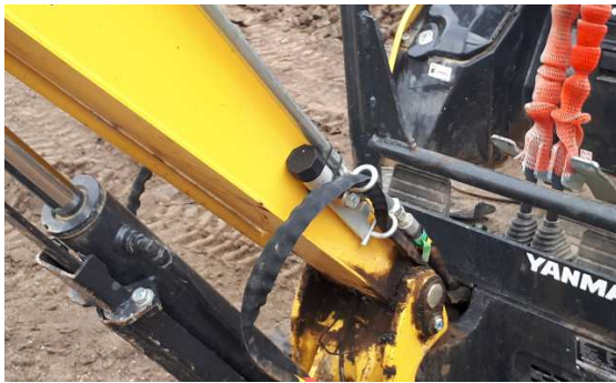
Figure 1: Fixing NaBi to construction equipment or refrigerator compressor
