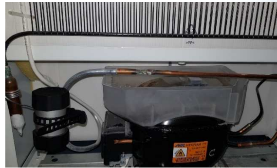
Figure 1: Fixing NaBi to construction equipment or refrigerator compressor
