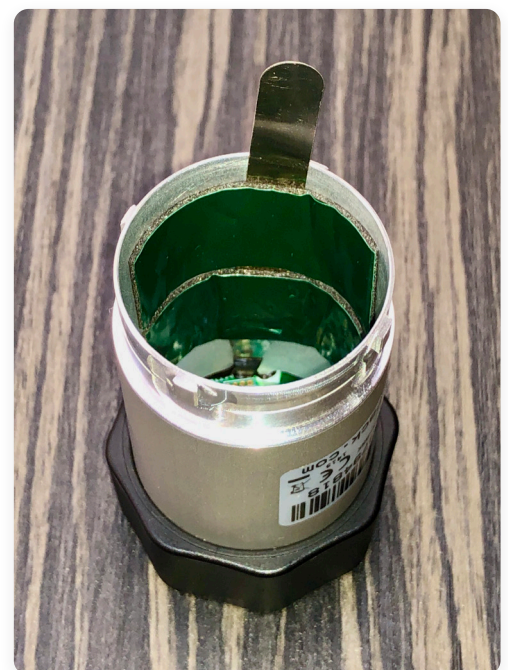
Figure 4: Placing a foam tape glued to the inside
